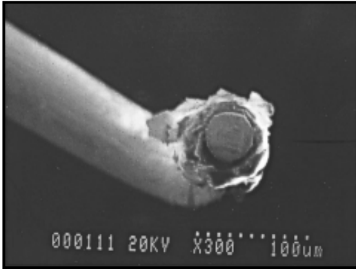
BEFORE – “Dirty” tungsten-rhenium probe tip.
