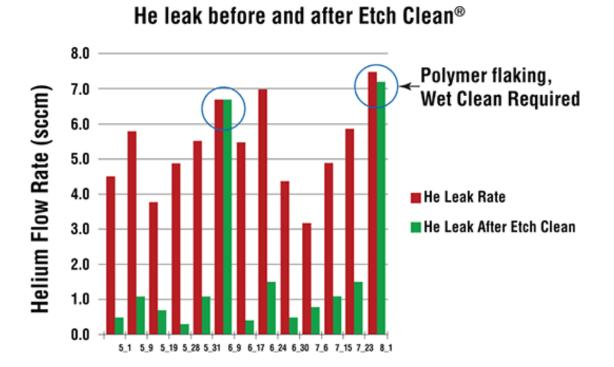
The maximum benefit from Etch Clean can be achieved when the wafer is cycled regularly as part of a preventative maintenance procedure. The Etch Clean process can be scheduled after wet clean or during other routine test procedures.
