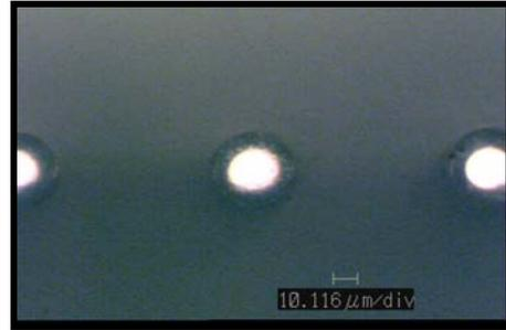
**Probe tips after 5 Probe Clean™ insertions.**
