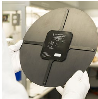
AMS200 multi-wafer with leveling, vibration and humidity is an ideal target for TEL Tracks. Maintaining these track tools requires well calibrated wafer handling as well as the monitoring of humidity in the chambers.
